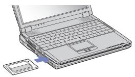
Gently push the card into the slot until the card is fixed into the connector.
